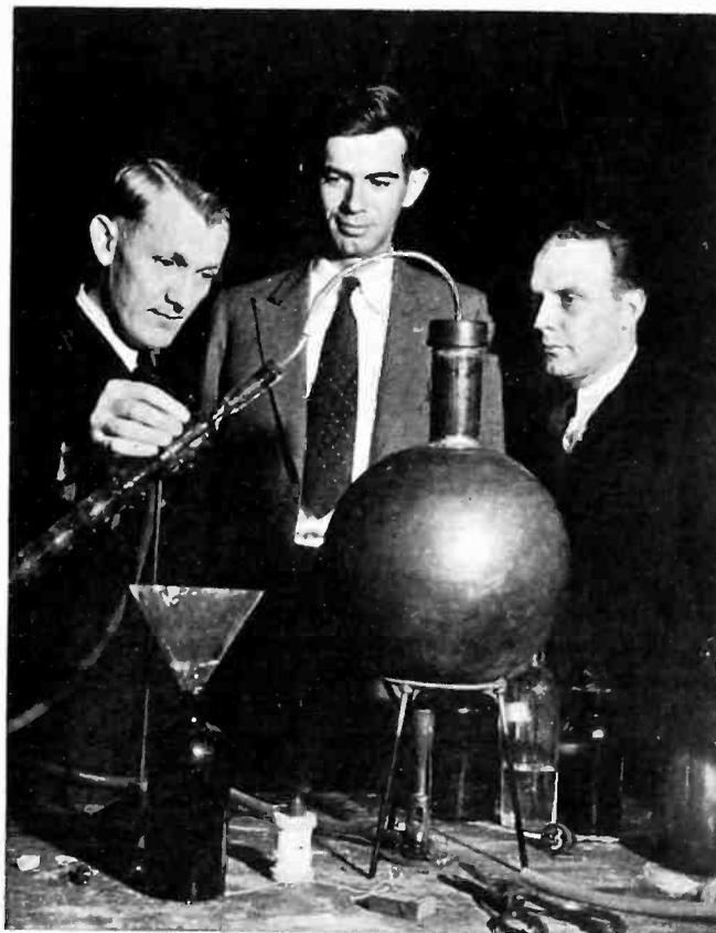
Dr. Charles C. Lauritsen of Caltech, shown with his associates Richard Crane and W. W. Harper, has succeeded in producing a new isotope of nitrogen having highly radio active properties by bombarding carbon with deuterons, or "heavy-water" nuclei. The apparatus shown is the first to produce a radio-active substance by a purely artificial technique.
