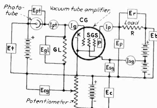
Fig. 1—Phototube amplifier circuit.
