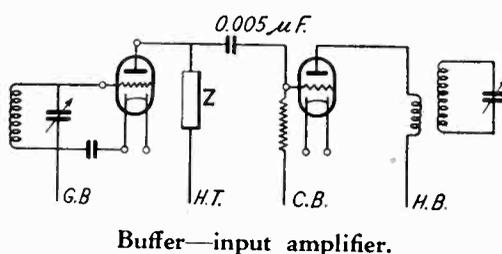
In the 200 kc. range, this system gives high amplification—up to 300 or more—and the input shunt resistance of the buffer tube is also very high.
