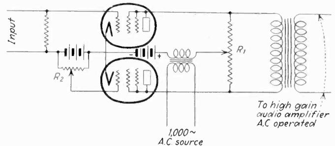
Fig. 8—Circuit for detecting and recording very small voltage changes.
