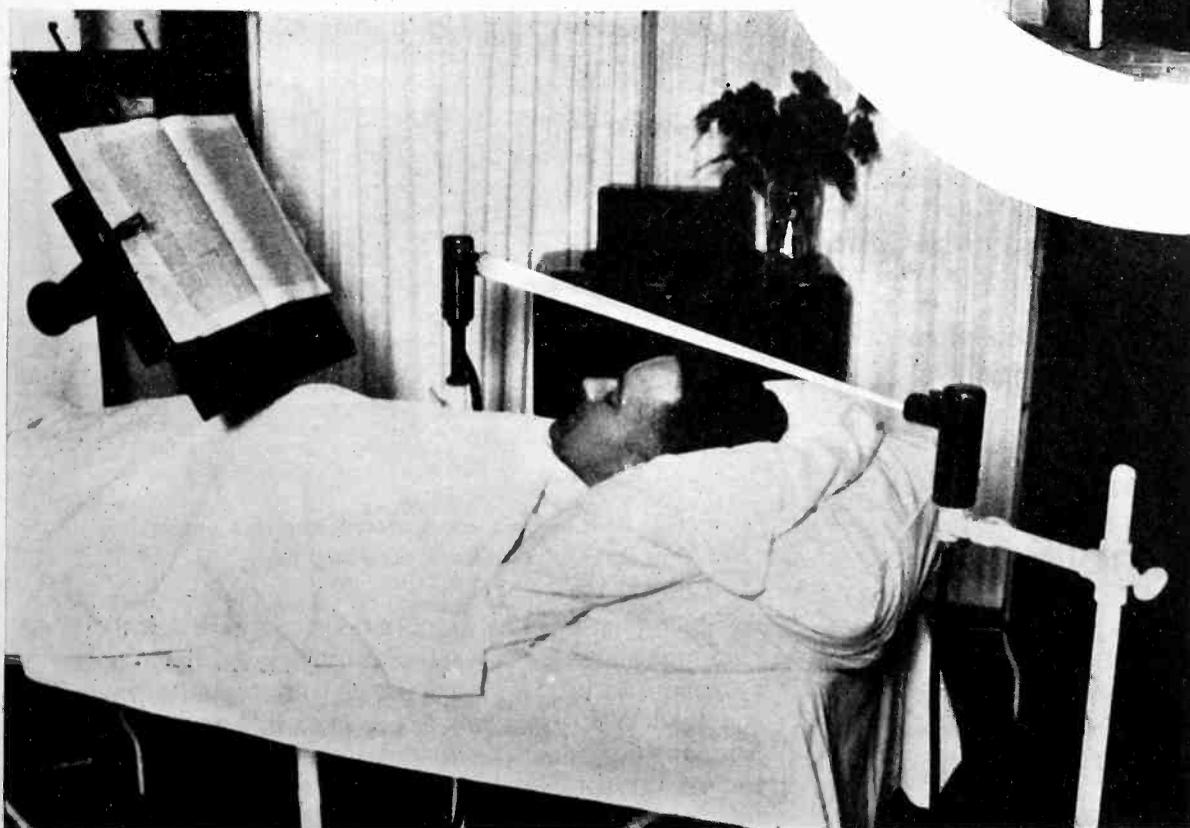
By means of this photo-cell combination, the totally-paralyzed boy has merely to move his head into the light-beam to turn the pages of the book. The mechanism goes through a sequence with book, radio, etc. These novel applications were developed by J. S. Doyle, electrical engineer, Interborough Rapid Transit Company, working with Dr. J. J. Moorhead, noted surgeon.
