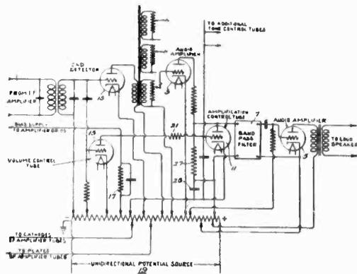
for controlling the range of frequencies to which the audio frequency amplifier is responsive. G. L. Beers, R.C.A. No. 1,961,329.
