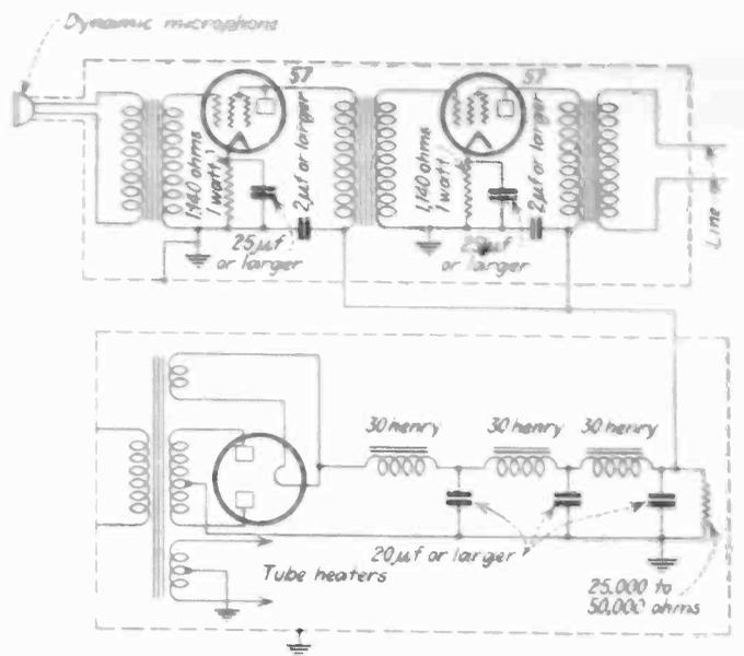
Fig. 1—A ribbon or dynamic amplifier for operation from a.c. supply
