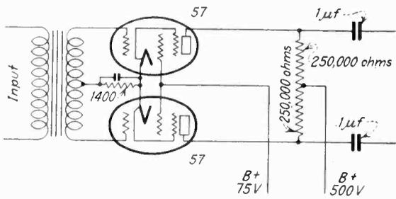
Fig. 6—Amplifier for high gain, low distortion, low noise and low hum.
