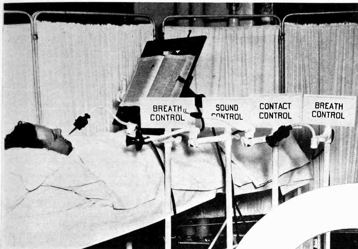
These various forms of control were developed for the use of a boy who is totally paralyzed from the neck down, so that he cannot move even a finger. But by touching his tongue to the electrodes leading to a "contact relay," or by blowing his breath or uttering a sharp sound, the book, radio, lights or call-bell can be manipulated.
