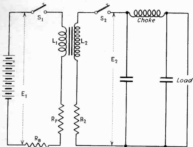
Fig. 1—Circuit for vibrator power supply.
