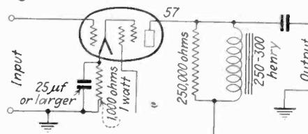
Fig. 5—Impedance coupled amplifier for high gain.
