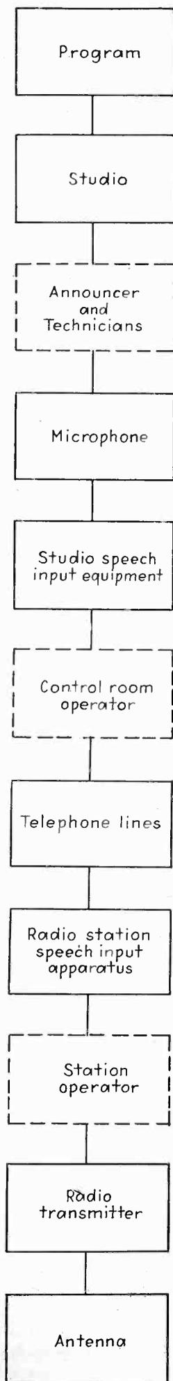
limitations. The long lines used for chain broadcasting are seldom better than 5,000-cycles on the high end and 80 to 100 cycles on the low. Many circuits will not deliver frequencies over 4,000. Here again better lines can be constructed, but line charges quickly become prohibitive. Even with their limitations, present line characteristics are better than the receivers.
