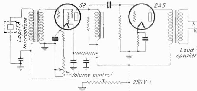
Fig. 4—Public address amplifier with an output of 3 watts operated from a lapel microphone.
